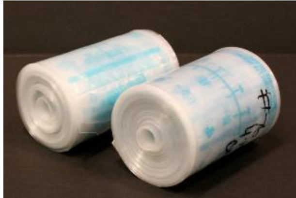
Figure 10: Liners Unevenly Rolled on a Non-Conforming Core (left); Liners Evenly Rolled on a Conforming Core (right) {Permission granted by Liz McCarthy (photographer)}
