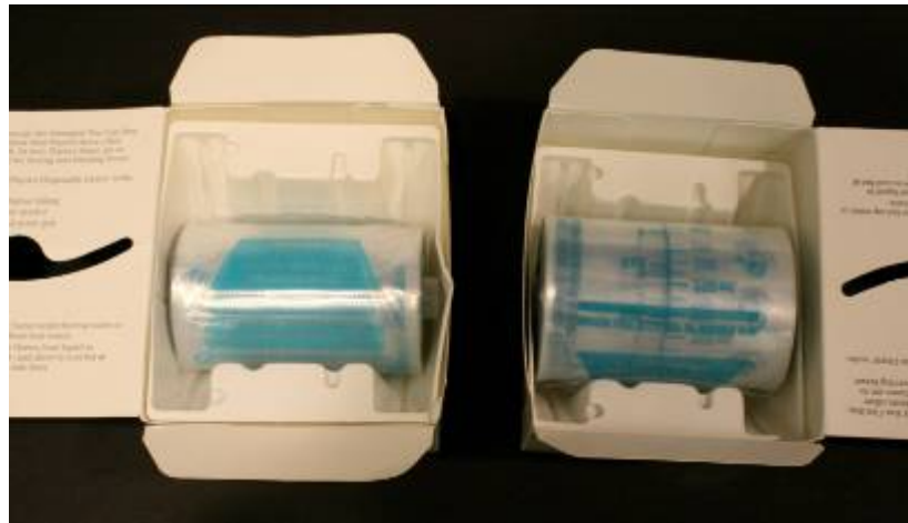
Figure 11: Unevenly Rolled Liners that Do Not Conform to Expectations (left); Evenly Rolled Liner that Conforms to Package Design (right) {Permission granted by Liz McCarthy (photographer)}
