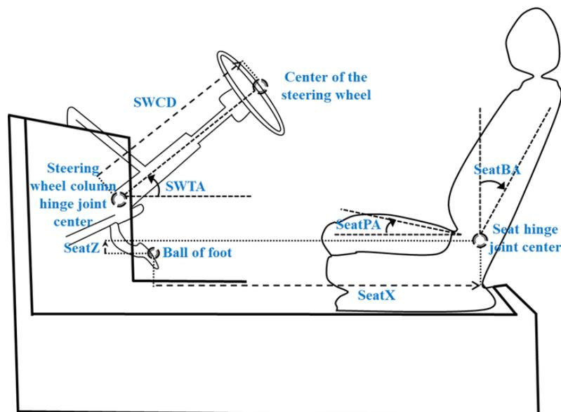
Figure 1. Variables representing the vehicle interior components setting
