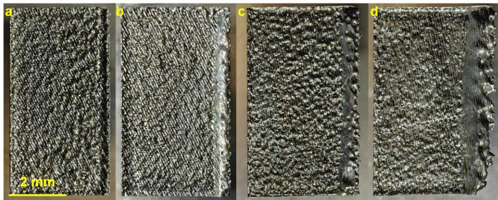
Figure 7. Surface quality variation of specimens under different overhang angle conditions: (a) 45^\circ ; (b) 50^\circ ; (c) 55^\circ ; (d) 60^\circ .
