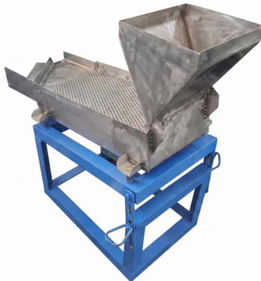
Figure 1. Laboratory-scale vibratory coffee sorting machine used in the experiment.
