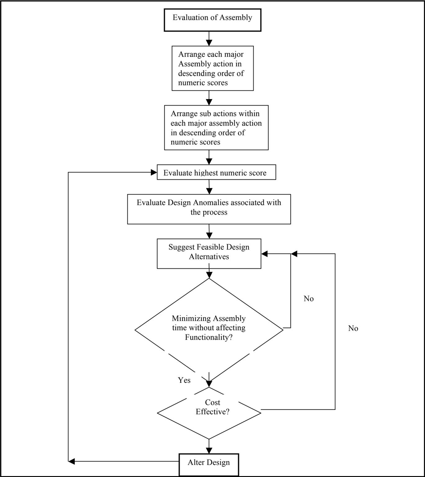
Figure 2: Methodology to enable design improvement for Product Assembly
