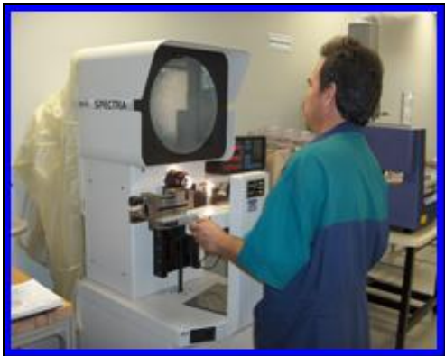
Figure 7. Measuring Tool against Drawing
