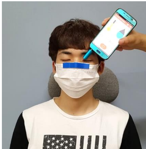
Figure 10. Humidity measurement wearing a half-face mask with the novel nose clip
